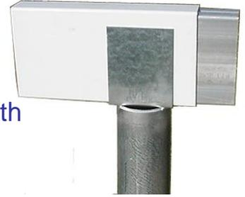
When placement of bottom beam is correct, place rail connector (A) inside post, over bottom carrying beam. It will be aligned so top cross beam will slide through (B). Slide filled cross beam through top holes, again leaving equal amounts protruding. If necessary, check for square. Ensure all beams extend equally beyond the posts before securing.
